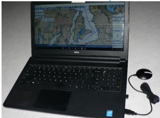
Dell Laptop with Windows 10 OpenCPN Chart Plotter Software USB GPS antenna (backup)
